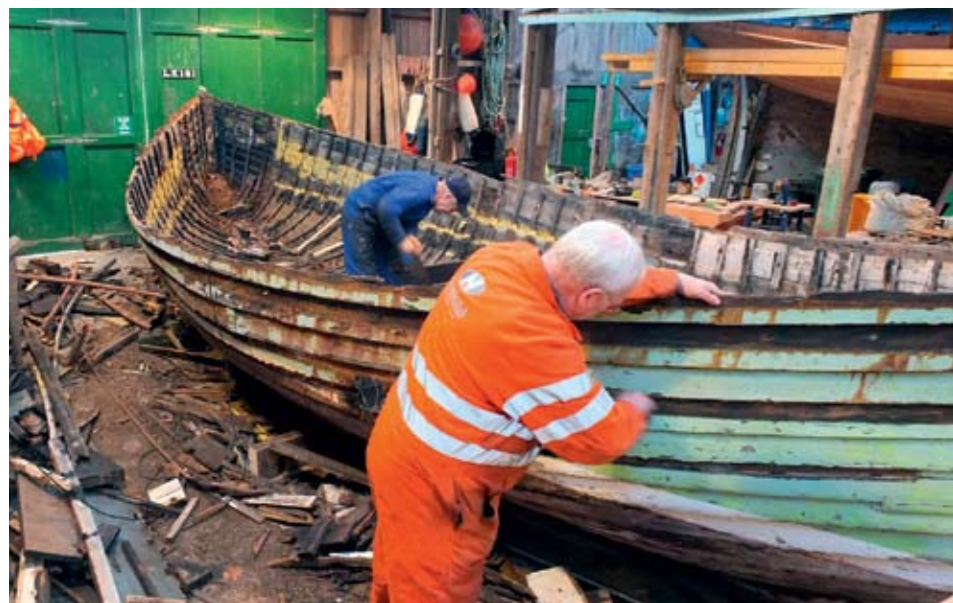
Jack Duncan (foreground) and Robbie Tait removing the later timber from No.6 lifeboat. The 1920s changes included a foredeck, different gunwales, rubbing strakes, engine beds, and a hefty stem and stern. The original 1899 timber is in very good order.
