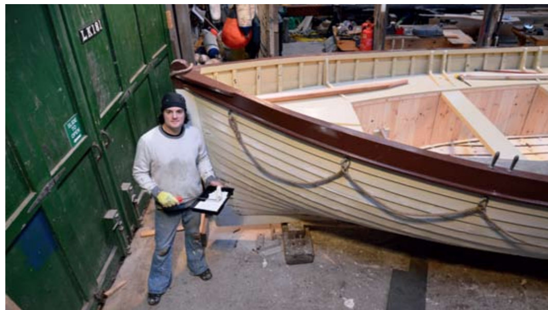
Museum volunteer Graeme Taylor has a special interest in White Star Line ships, and his dedication in preparing and painting R.M.S. Oceanic 's lifeboat was indispensable to the project. The original colours were reinstated; cream hull, brown gunwales, buff inboard.
